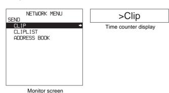
The SEND CLIP screen appears, showing the currently selected destination host name, the transfer target clip, and its duration.
